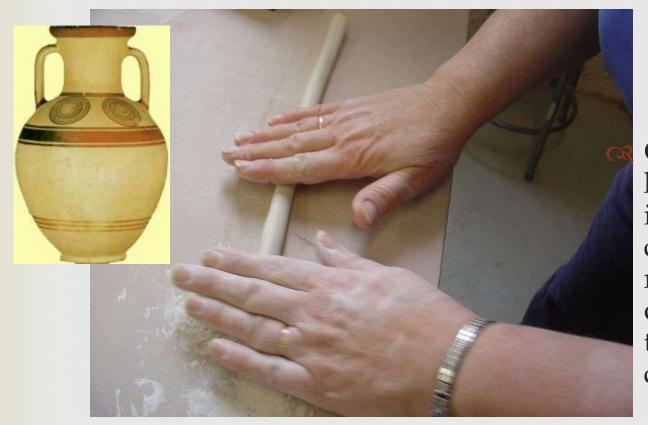
COILING is an ancient hand building method in which walls are constructed with and rolled, rope-like pieces of clay. The joints are then smoothed over to create one solid piece.
